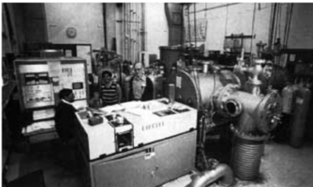
Fenn's "big leak" molecular-beam system, with two 32 inch diffusion pumps and one 16 inch "jet Booster Pump," after it was moved from Princeton to Yale. Fenn, standing at center, is accompanied by two postdoctoral fellows, S.B. Ryali, also standing, and S.P. Venkateshan, sitting. © The Nobel Foundation 2002.
